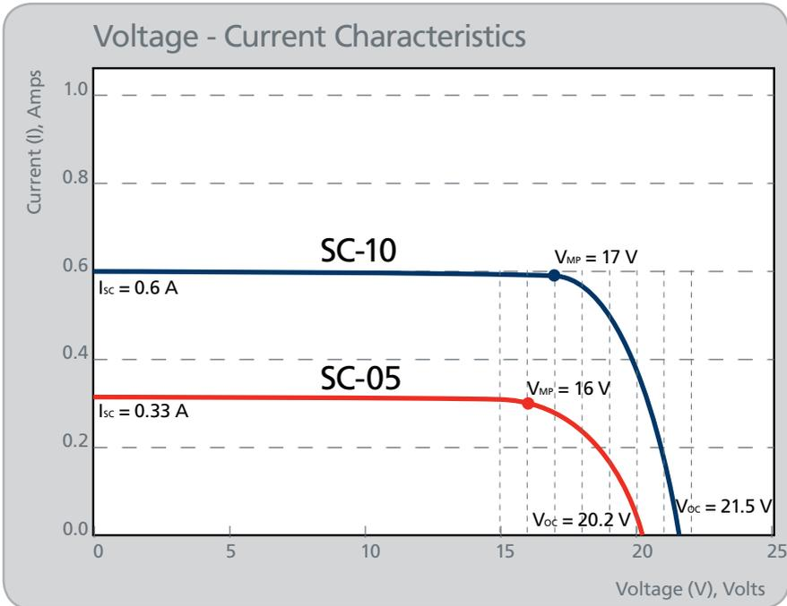
Fig. 1. Voltage versus Current characteristics.
